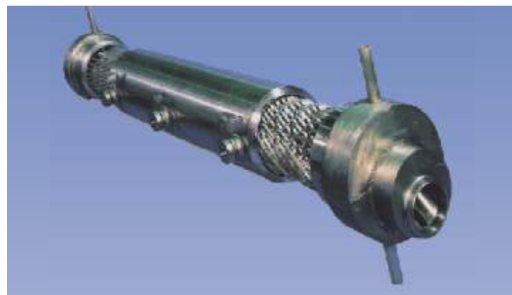
Figure 7 - Pre-assembly of a round SMR mixer-reactor designed for 250 bar / 300 °C in a gap-free fixed tube-bundle design used as a polymer melt cooler.
