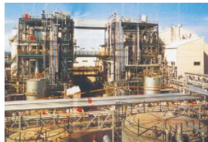
Figure 11 - Plants for the production of 30,000 t/year of crystal polystyrene (left) and 35,000 t/year of high impact polystyrene (right) using the SDS process (Sulzer - Dainippon Ink & Chemicals - Sumitomo).
