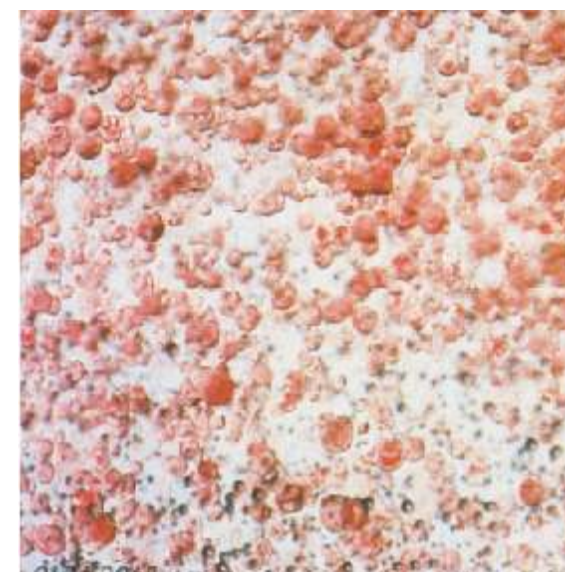
Figure 4 - Droplet pattern after SWV disperser. Dispersed phase = kerosene dyed red, continuous phase = water.
