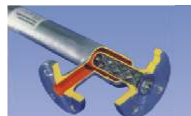
Figure 8 - SMXL monotube mixer heat exchanger flows through the mixing elements. The heating or cooling media flows through the jacket, separated from the product.
