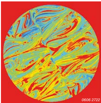
Laminar mixing in the Sulzer SMX™ mixer shown with Laser Induced Fluorescence
